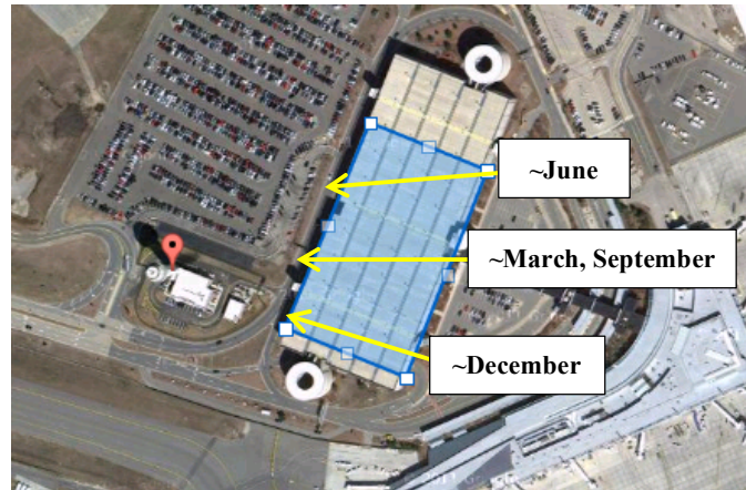
Figure 20. Approximate predicted locations and movement of glare on PV array at various times of the year.
